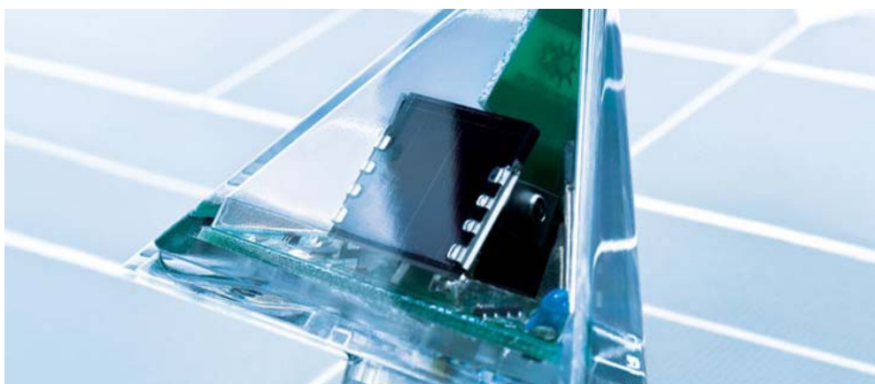
MLD Sensor Used on site to orientate the system
